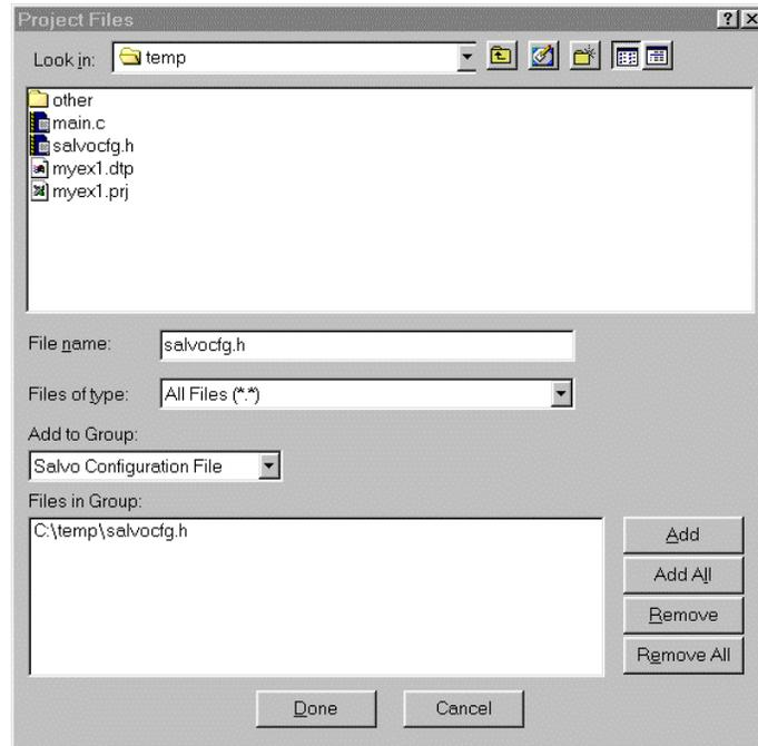
**Figure 12: Adding the Configuration File to the Project**
