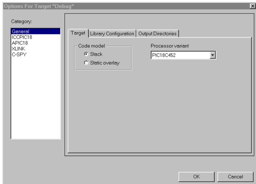
**Figure 4: Setting the Code Model and Processor Variant**
