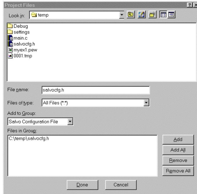
**Figure 16: Adding the Configuration File to the Project**
