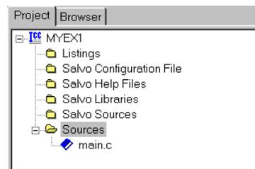
Figure 8: Project Manager Window with Project-Specific Source Files
