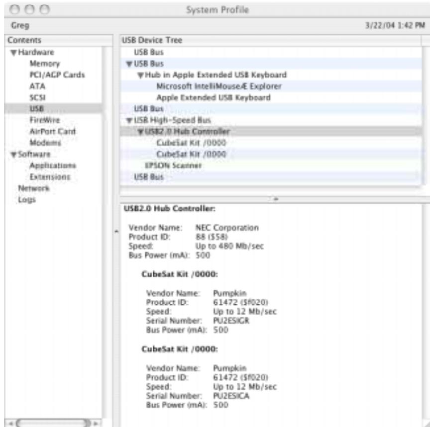
**Figure 20: Two CubeSat Kits Connected over USB**
