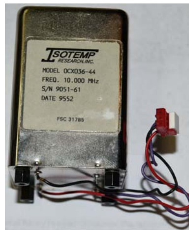
Figure 3: IsoTemp OCXO36-44, the "original" Option 115 OCXO for Model 3xxx frequency counters
