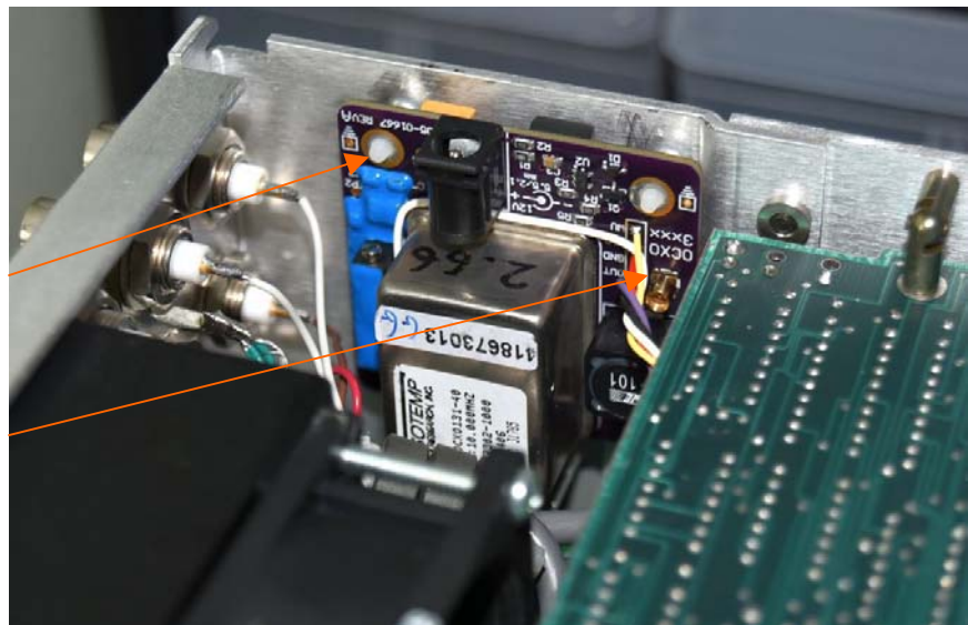
Figure 7: OCXO PCB assembly installed in DS345
