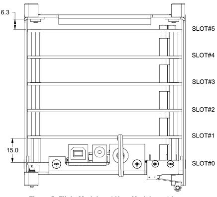
Figure 5: Flight Module + 4 User Modules + 1 Low-Profile User Module
