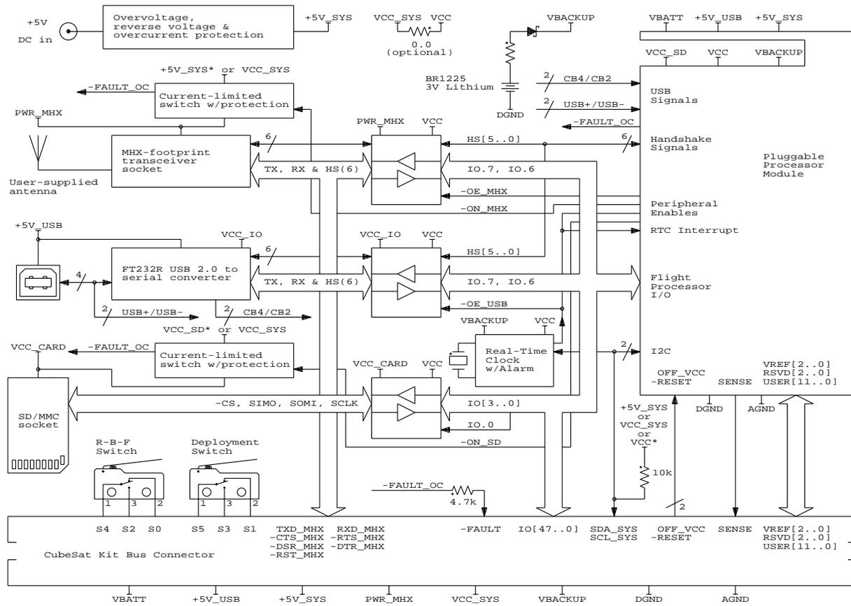
\*: Default configuration, selectable via 0 Ohm resistors / jumpers.
